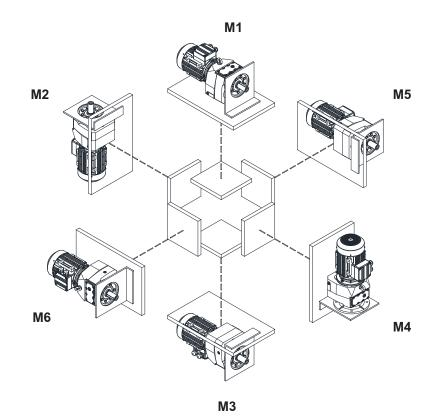
Indicated mounting positions are determined as reference directional position of the gearbox. Mounting surfaces are not binding.
