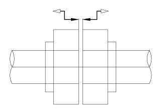
**7.3.2**- When installing the coupling, please observe the maximum permissible axial misalignment.
