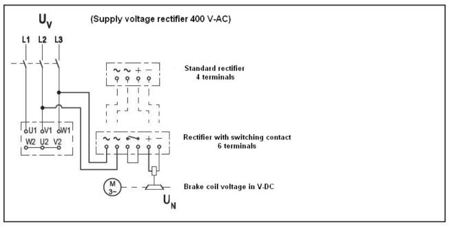
Supply: Phase-Phase Half-wave rectifier
